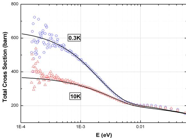
Fig. 2. (Color online) Comparison of the calculated total cross sections of methane at 0.3 K and 10 K, with measured points [9].
