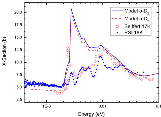
Fig. 4. (Color online) Calculated total cross sections of ortho- and normal-deuterium at 18 K, compared with the experimental data from Refs. 18 and 19.
