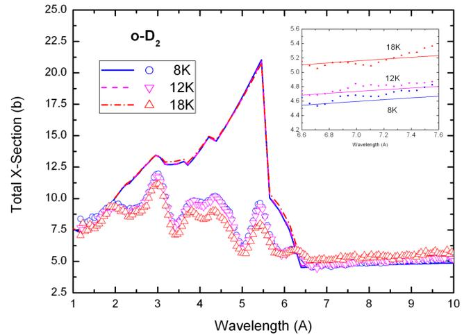
Fig. 3. (Color online) Calculated total cross section of solid  $o\text{-D}_2$ , compared with experimental data from [17,18]. The inset shows that comparison beyond the first Bragg peak.
