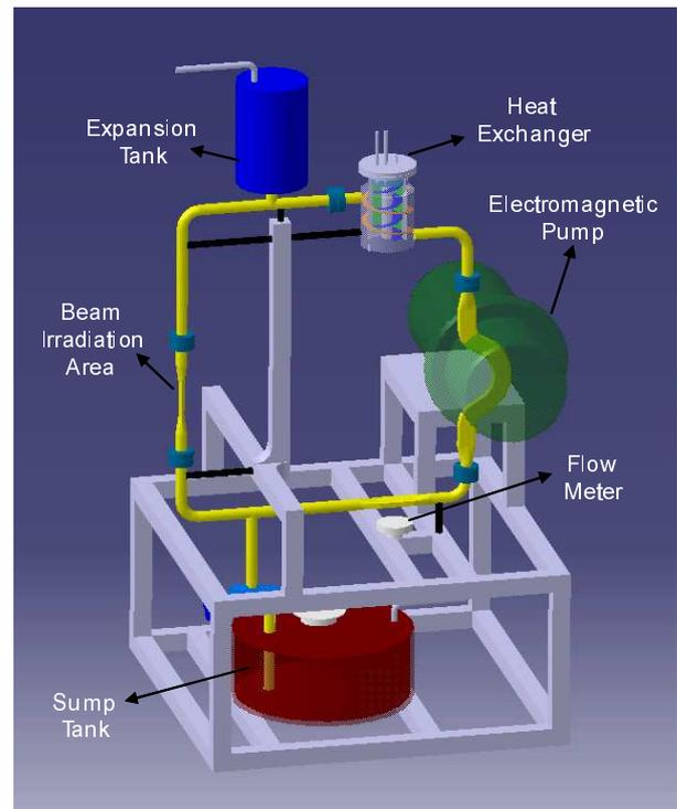
Fig. 3. (Color online) Liquid Pb target system.
