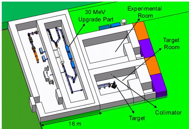
Fig. 2. (Color online) TOF facility to be constructed in the second phase.
