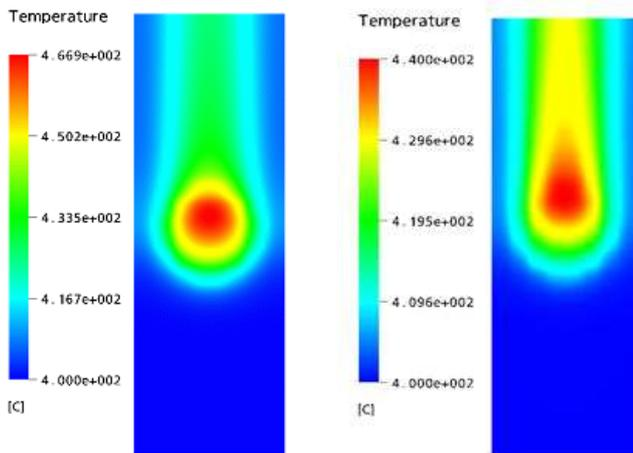
Fig. 4. (Color online) Temperature distributions of the Mo outer surface (left) and Pb surface contacted by Mo wall (right) at a velocity of 2 m/s.
