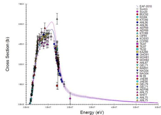
Fig. 4. (Color online) Cross section data for  $^{54}\text{Fe}(n,p)^{54}\text{Mn}$  in the EAF-2010 library, the dotted line indicates the library uncertainty. The points represent measurements from EXFOR.
