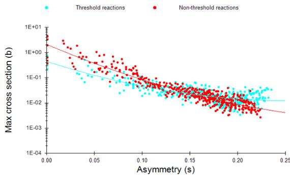
Fig. 5. (Color online)  $\sigma_{\max}(s)$  for all (n,p) reactions in EAF-2010. Threshold and non-threshold reactions are distinguished. Reactions with targets  $A < 20$  are excluded.
