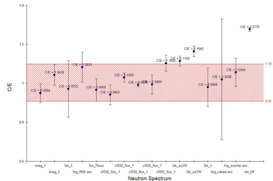
Fig. 3. (Color online) C/E data for  $^{54}\text{Fe}(n,p)^{54}\text{Mn}$  measured in various neutron spectra. The band indicates the uncertainty in the library.
