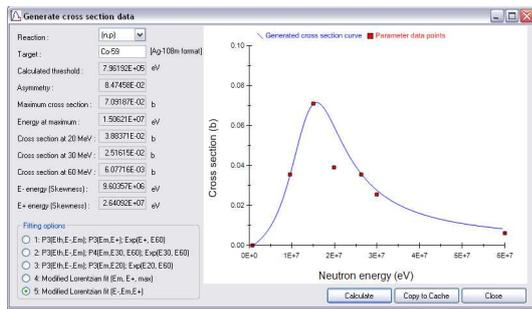
Fig. 2. (Color online) Generate cross section data tool for threshold reaction types, implemented in SAFEPAQ.
