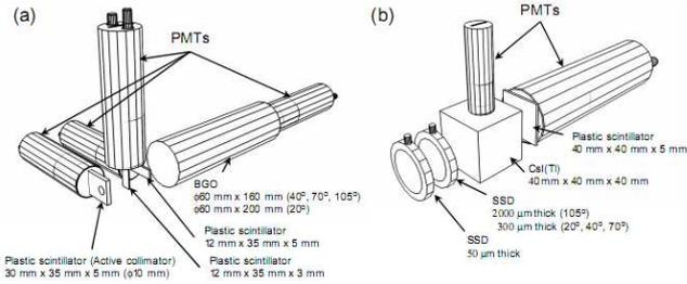
Fig. 2. Layout of the spectrometers. (a) high-energy module, (b) low energy module.
