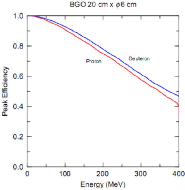
Fig. 4. (Color online) Peak efficiency of the BGO detector.
