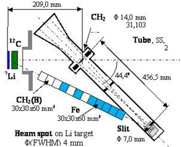
Fig. 1. (Color online) The experimental arrangement of the proton-recoil- telescope experiment.
