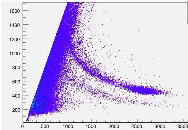
Fig. 3. (Color online) The  $(\Delta E1+\Delta E2) \times (\Delta E1+\Delta E2+E)$  pulse-height matrix from the  $\text{CH}_2$  expositon.
