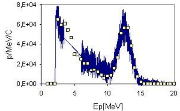
Fig. 5. (Color online) The measured proton recoil spectrum (line) compared with the MCNPX simulation (squares).
